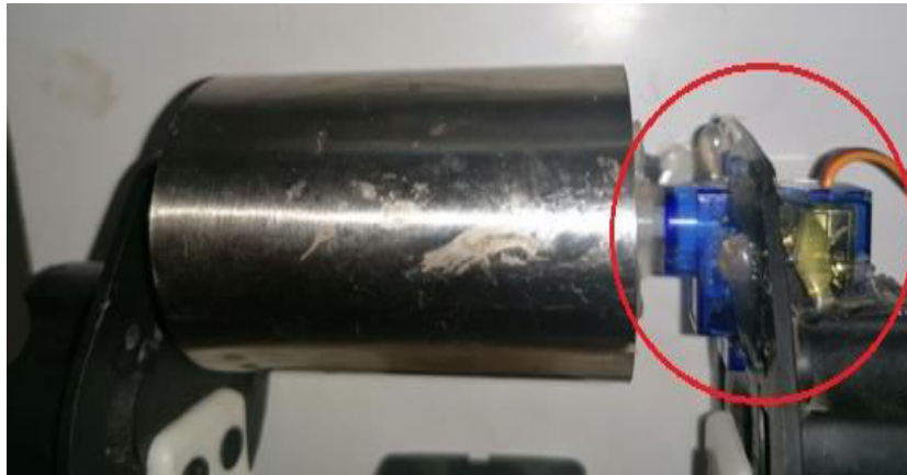
Fig. 9 Installing the SG990 servo motor
