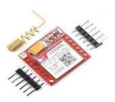
A GSM modem or GSM module is a device that uses GSM mobile telephone tech- nology to provide a wireless data link to a network. GSM modems are used in mo- bile telephones and other equipment that communicates with mobile telephone networks.
