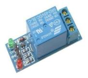
A power relay module is an electrical switch that is operated by an electromagnet. The electromagnet is activated by a separate low-power signal from a micro con- troller. When activated, the electromagnet pulls to either open or close an electrical circuit.
