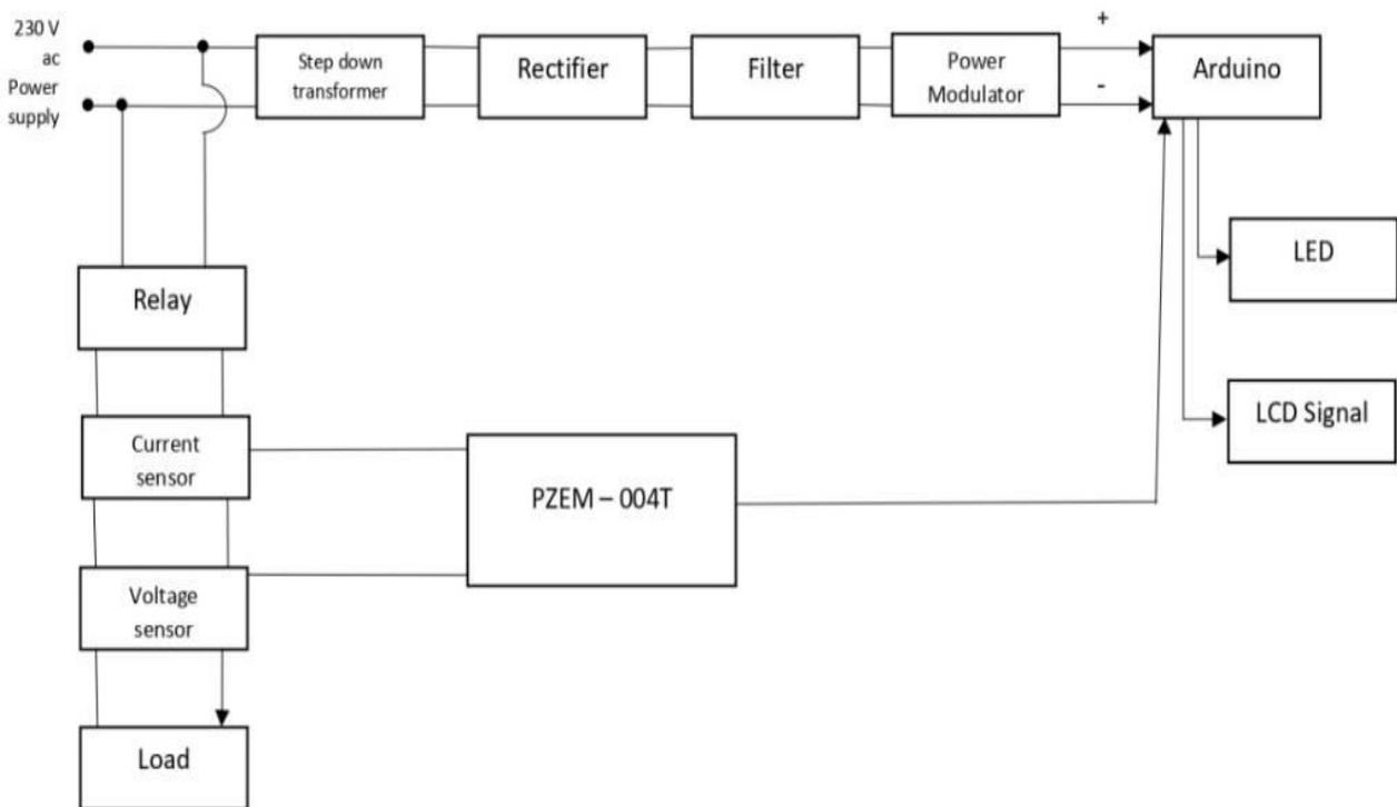
**Fig. 1:** Block diagram of the proposed methodology
