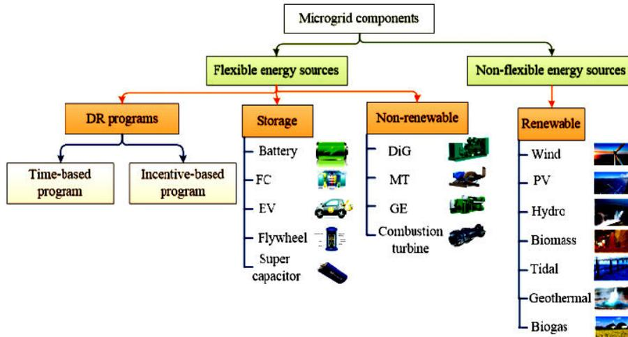
Figure 1: Microgrid Component
