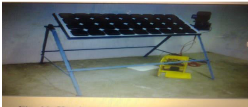
Fig.2 Sample PV panel Assembly
