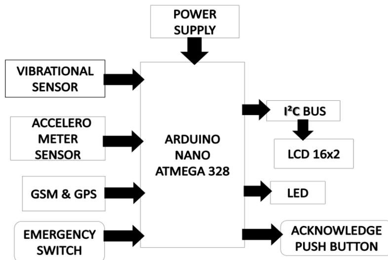
Fig 2. Hardware Block Diagram.
