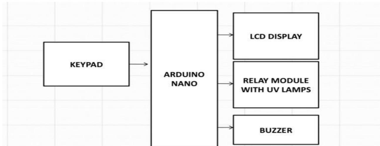
Fig.1 Block diagram
