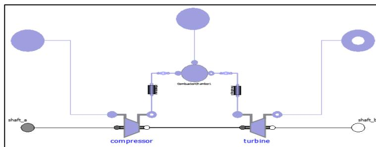
Fig. 5: The Single Shaft Gas Turbine model
