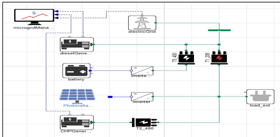
Fig.1:Micro-Grid Integrated System Model.
