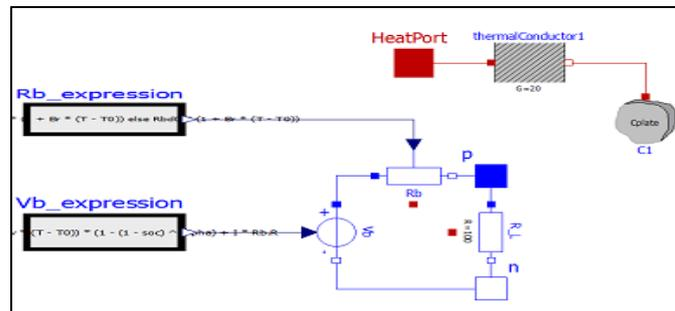
Fig .4: Battery Modelica diagram
