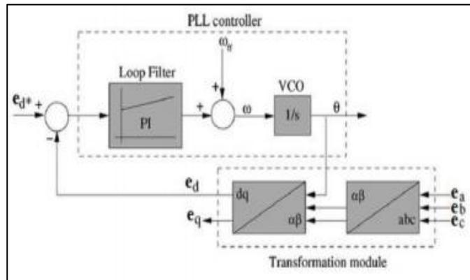
Fig .8: Basic structure of a PLL system for grid synchronization
