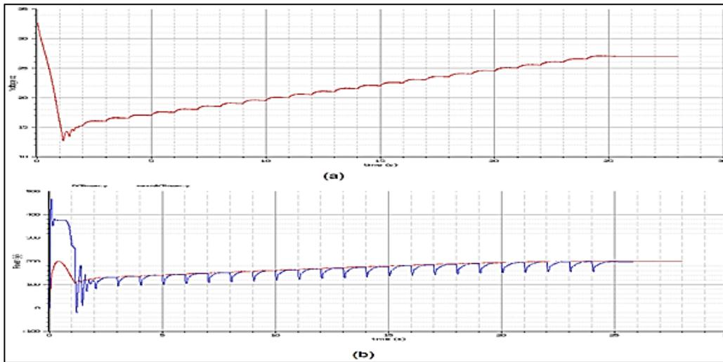
Fig.10: PVnverter1phSynch simulation results: (a) PV array voltage, (b) input and output power
