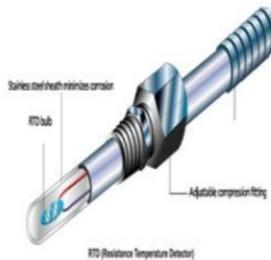
Resistor Temperature Detector (RTD)
