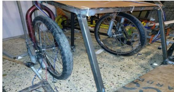
Fig.(d) Hardware design of wheelchair
