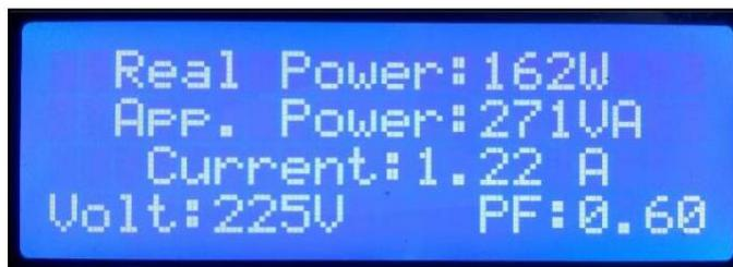
Fig 7: Load condition before power factor correction
