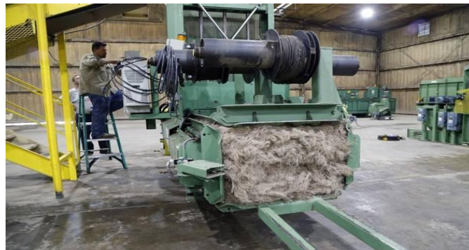
Fig.4 Kenaf fibre extracting machine
