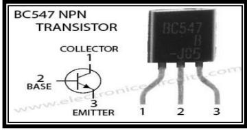
Fig no.6 Transistor BC547
