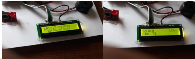
Figure.15:(a) GPS co-ordinates displayed on LCD (b)Heartbeat readings displayed on LCD
