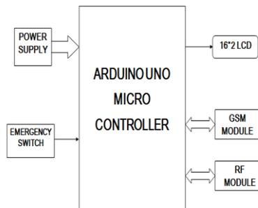
Figure.2 Block diagram of Receiver section
