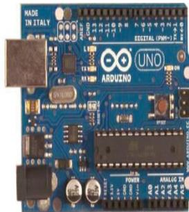
Figure.4 Arduino Uno microcontroller
