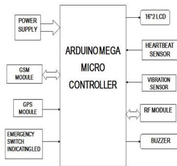
Figure.1 Block diagram of Transmitter section
