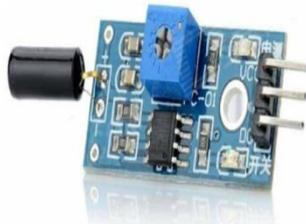
Figure5. Vibration sensor
