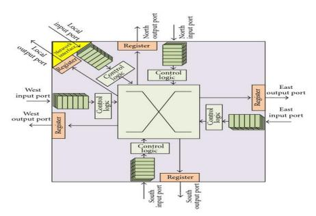
Figure 2: Typical NoC router architecture
