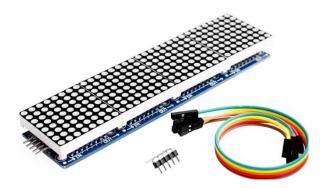
A single matrix display is made up of 8 by 8 LEDs. It means 8 rows and 8 columns of LED which makes it 64 LEDs in one block. So in total, there are 48 columns and 8 rows of LEDs. All LEDs are Red in color.
