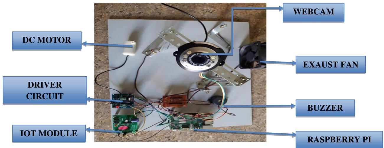
*Figure 1.2. Working kit for the Proposed model.*
