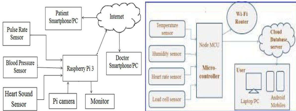
**Fig. 1: Block diagram of animal health monitoring system.**
