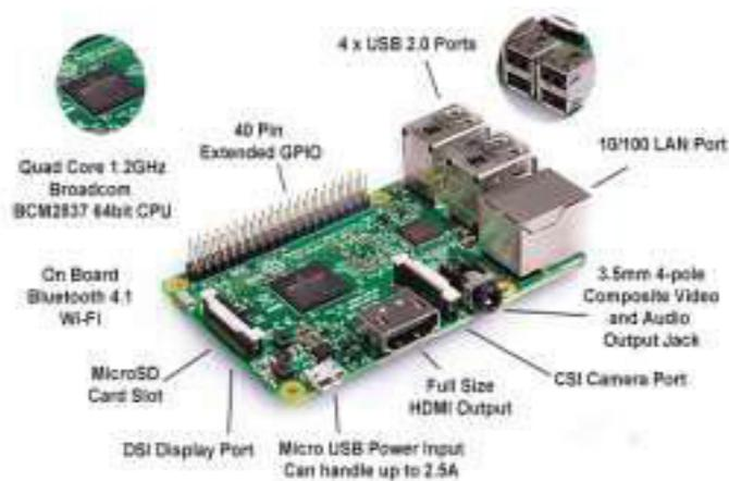
Fig. 2: Raspberry pi3 (top view)
