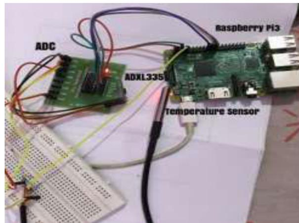
**Fig. 3: Interfacing diagram of Temperature sensor and ADC with RPi3.**
