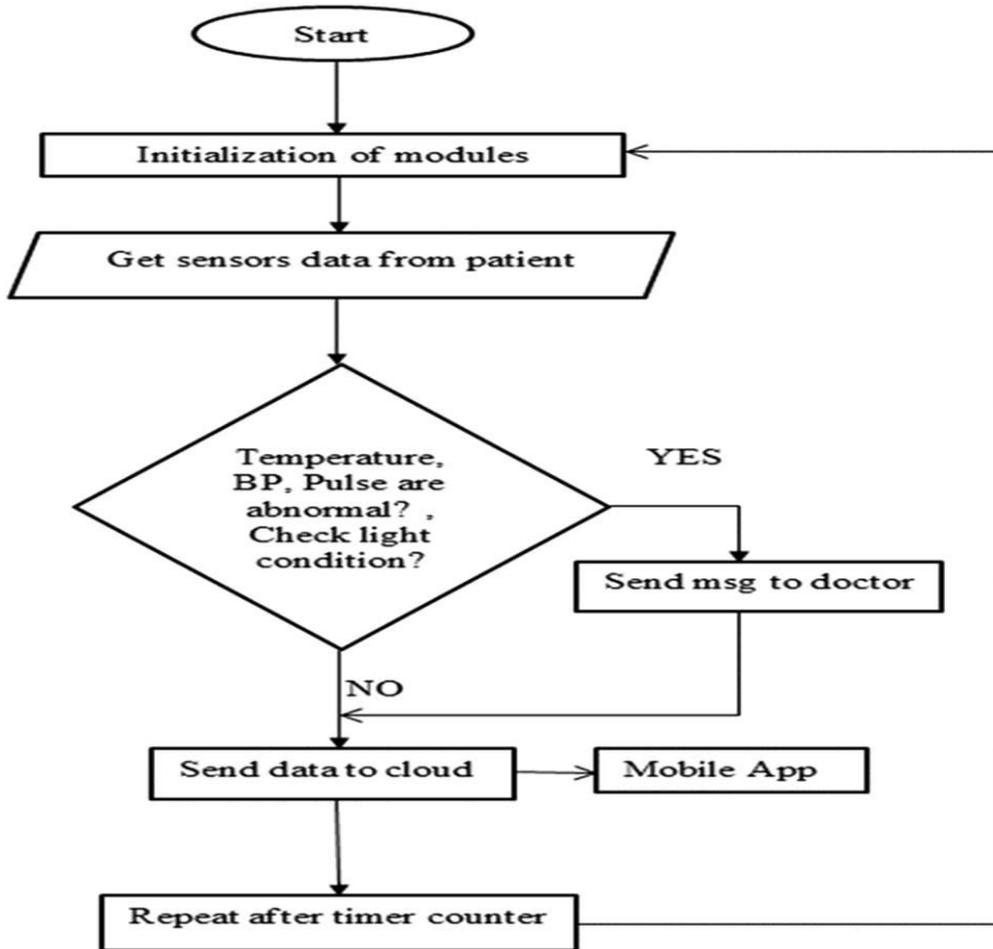
Fig. 5: Flow Diagram of the IoT based Smart Animal Health Monitoring System
