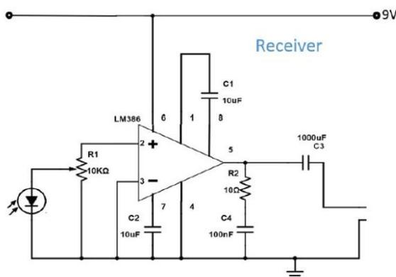
Fig.3 Proposed System Receiver Circuit
