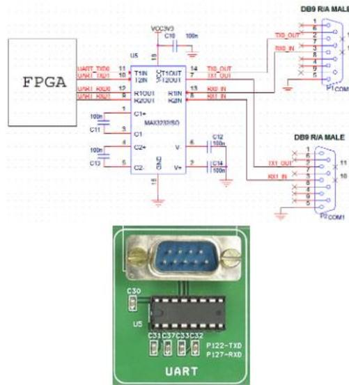
Fig.8RS232 – Interfacing Module Circuit
