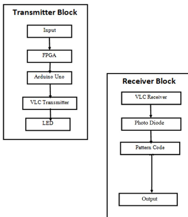
Fig.4Proposed System Block Diagram
