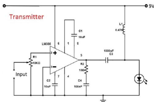
Fig.2 Proposed System Transmitter Circuit
