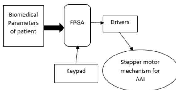
Figure 1. Block diagram of Automatic Anesthesia Injector
