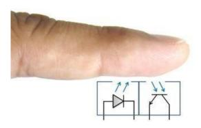
This sensor is based on the principle of photoplethysmography (PPG) which is a non-invasive method of measuring the variation in blood volume in tissue using a light source and detector. Change in blood volume is synchronous to heartbeat. Transmittance and reflectance are two basic types of photoplethysmography.
