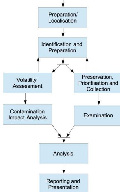
Figure 3: SCADA Incident Response and Forensic Process
