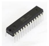
16f877a is one of the picmicro family microcontrollers. It uses a flash memory technology so it can be write and erase easily. It has large programming memory. It has 368 bytes of RAM. It has 256 bytes of EEPROM data memory and also it is self-programming. Its operating voltage is 4.0-5.5v, operating speed is 20MHZ.
