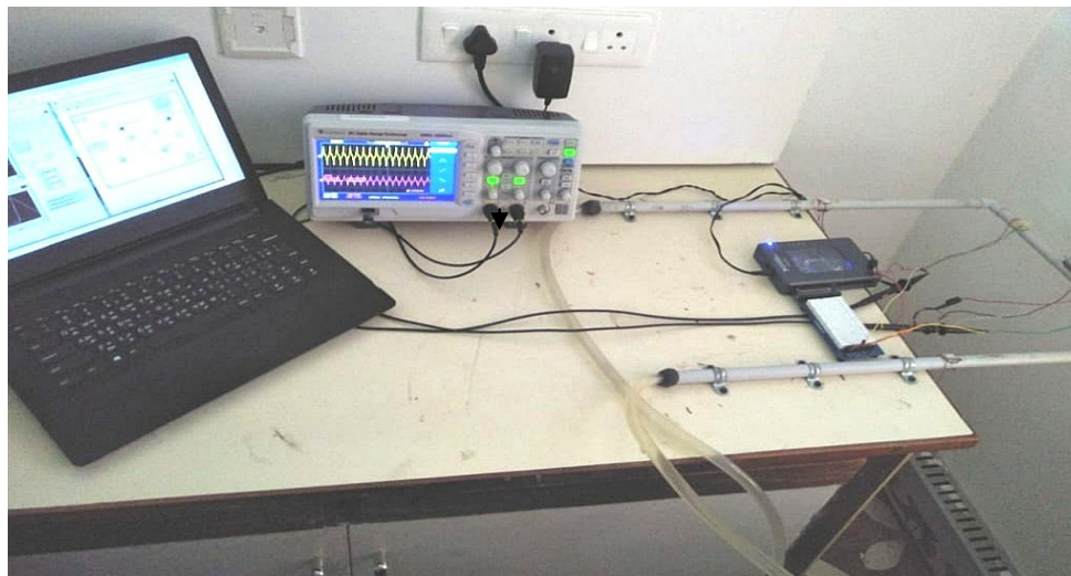
FIG-4 EXPERIMENTAL SETUP OF SINGLE U-TUBECORIOLIS MASS FLOWMETER
