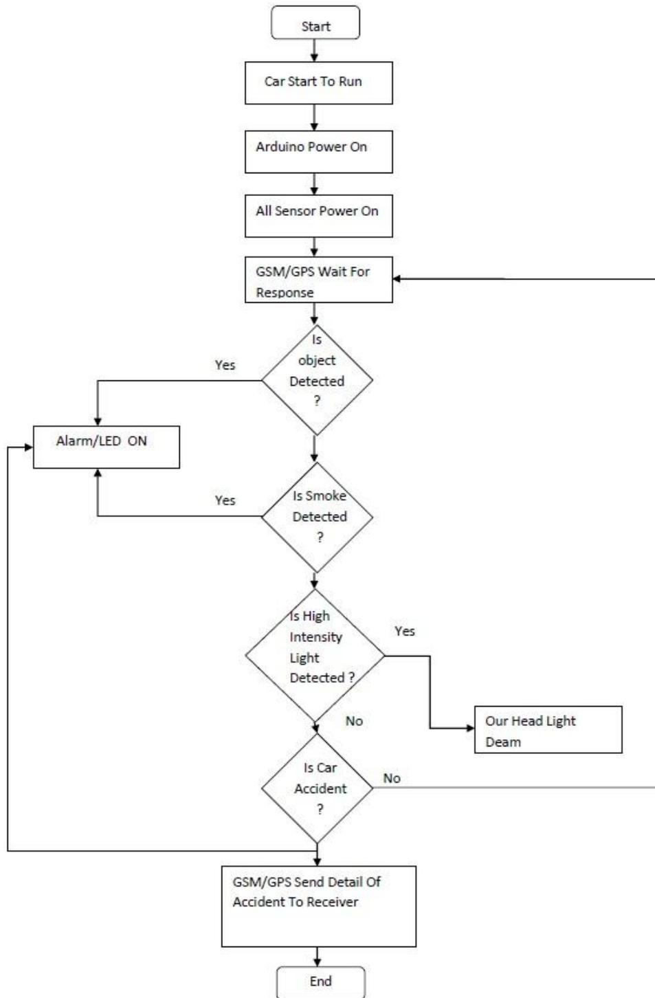
Fig. 2 Flow chart for Operation
