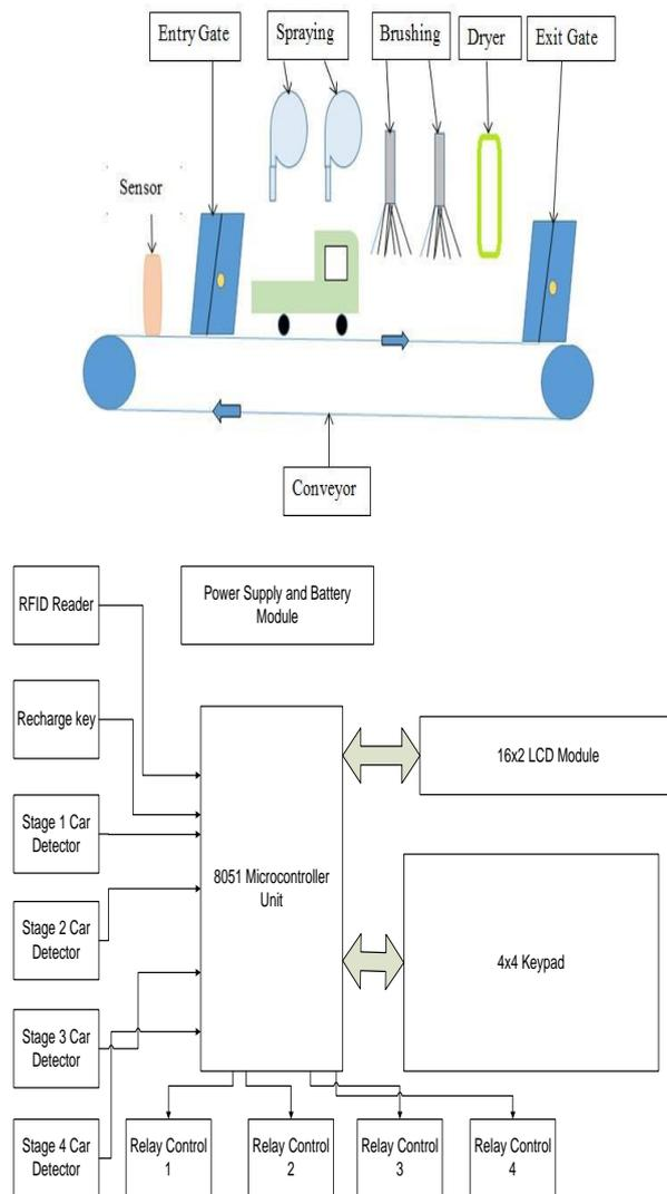
Fig.1: Block diagram of Automatic car washing system
