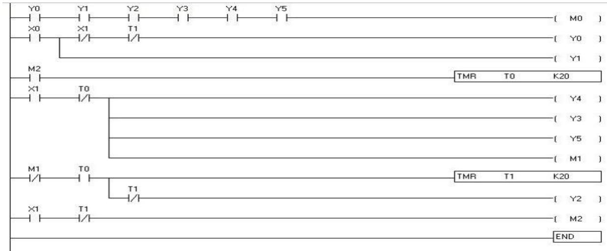
Fig 6 PLC ladder diagram for automatic bottle filling
