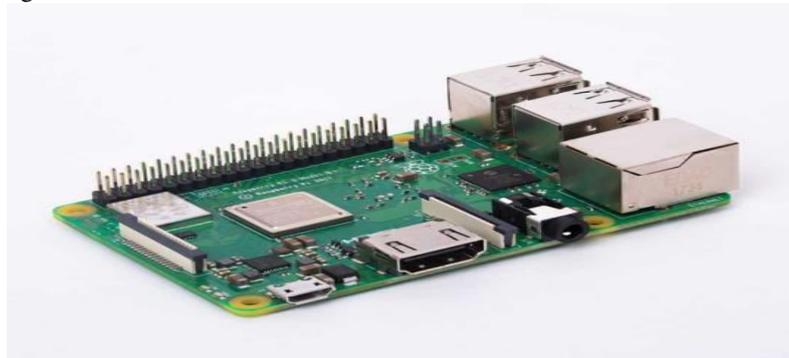
Fig.1. Hardware kit of raspberry pi 3B+
