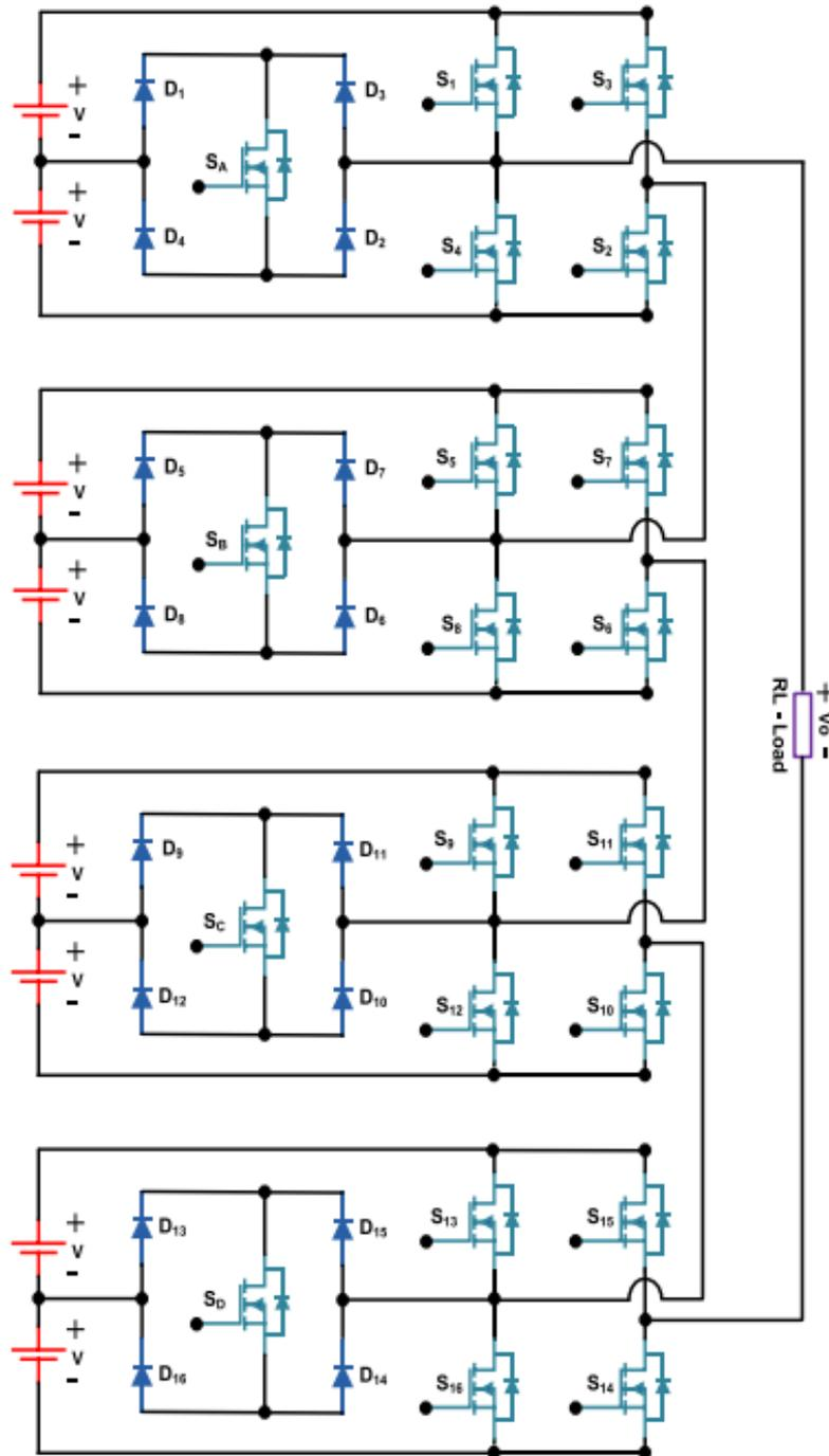
Fig 3. Proposed 17-level symmetric MLI
