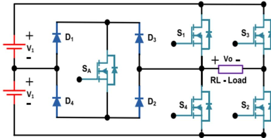
Fig.2. Basic Hybridised H-bridge topology.
