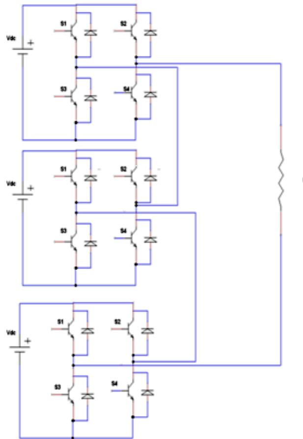
Fig 1. Circuit diagram of existing system
