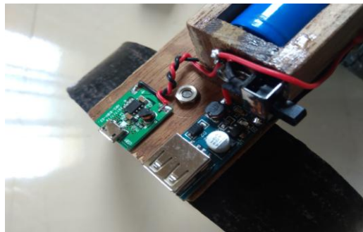
Figure 2 Step up converter DC-DC & TP4056 charging circuit.
