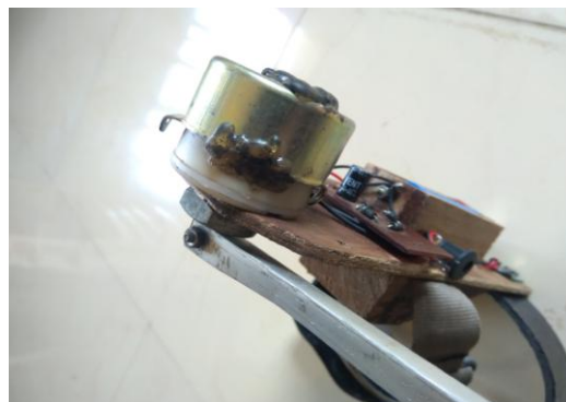
Figure 3 AC motor fused with geared box to work as generator.
