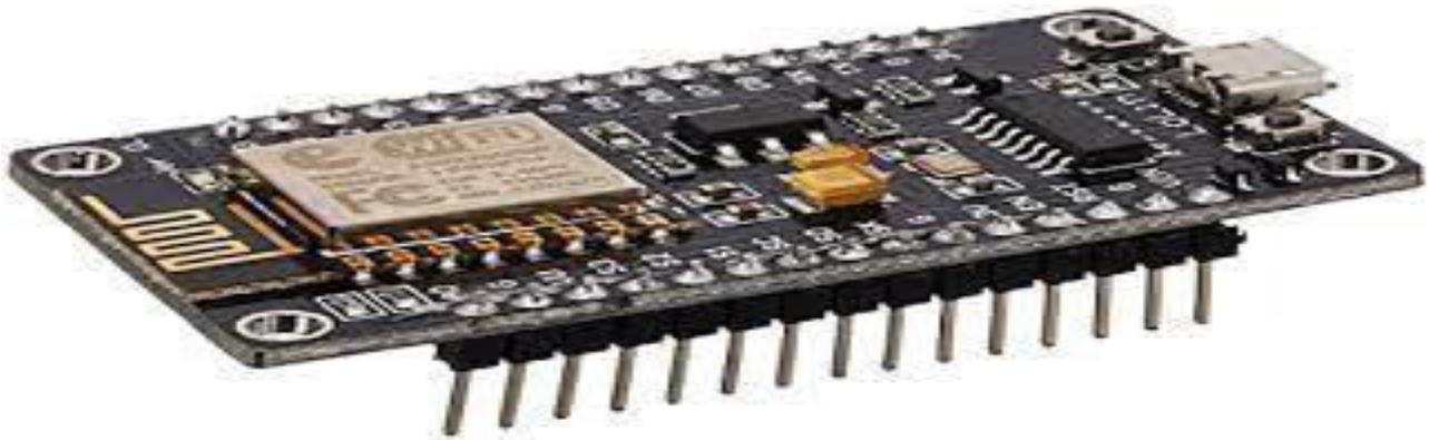
Fig -2: NodeMCU (ESP8266) Development Board
