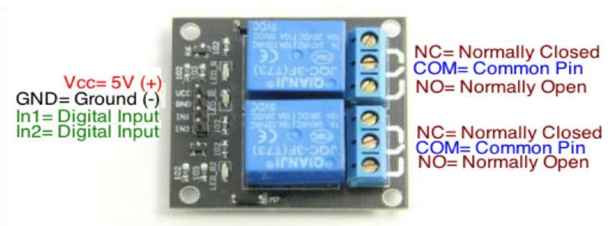
**Figure 5** 2-Channel Relay Mode
