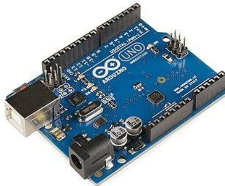
**Figure 6** Arduino UNO Microcontroller
