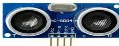
Figure 3 Ultrasonic Sensor
