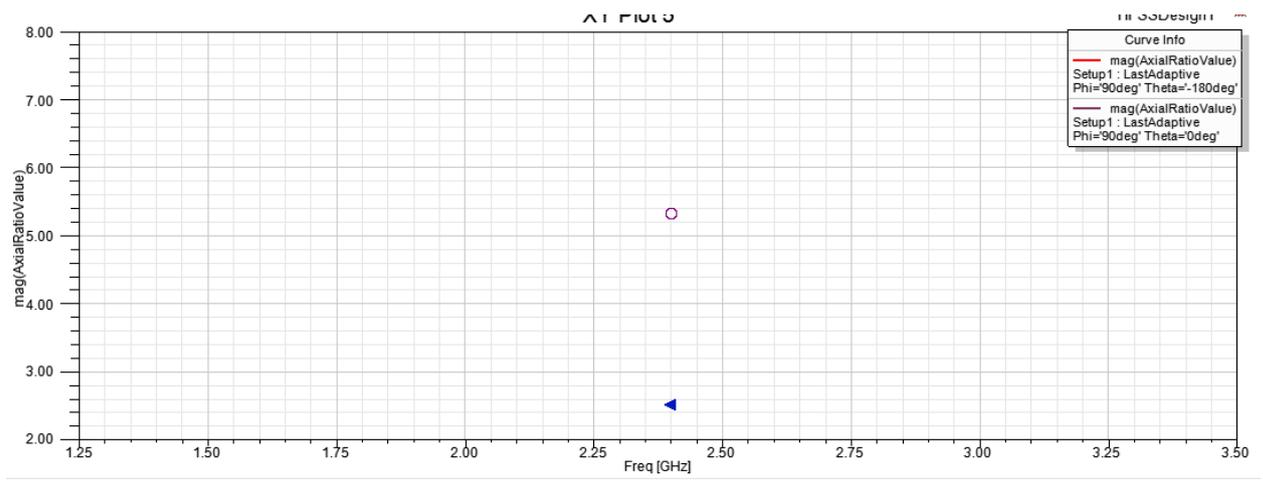
Axial ratio for proposed antenna with DGS
