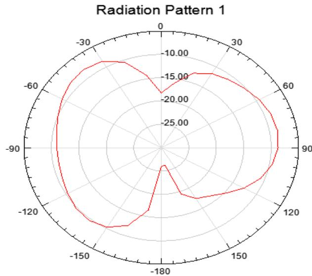
**Radiation pattern for proposed antenna with DGS**
