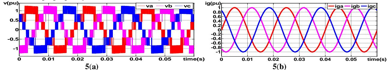
Fig.5. (a)Balanced 3-ph 7-level H-bridge inverter voltages  $v_a, v_b, v_c$ ; (b)Balanced grid currents  $i_{ga}, i_{gb}, i_{gc}$
