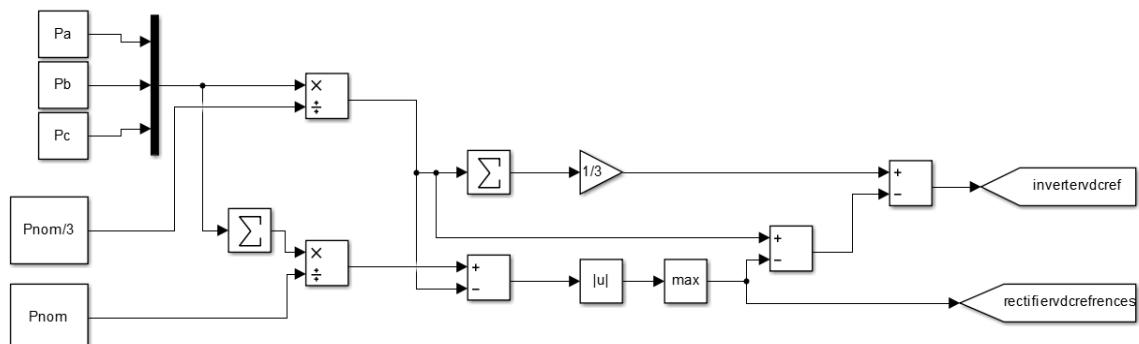
**Fig.4 control scheme of proposed systems for generating the voltage references for direct axis current**
