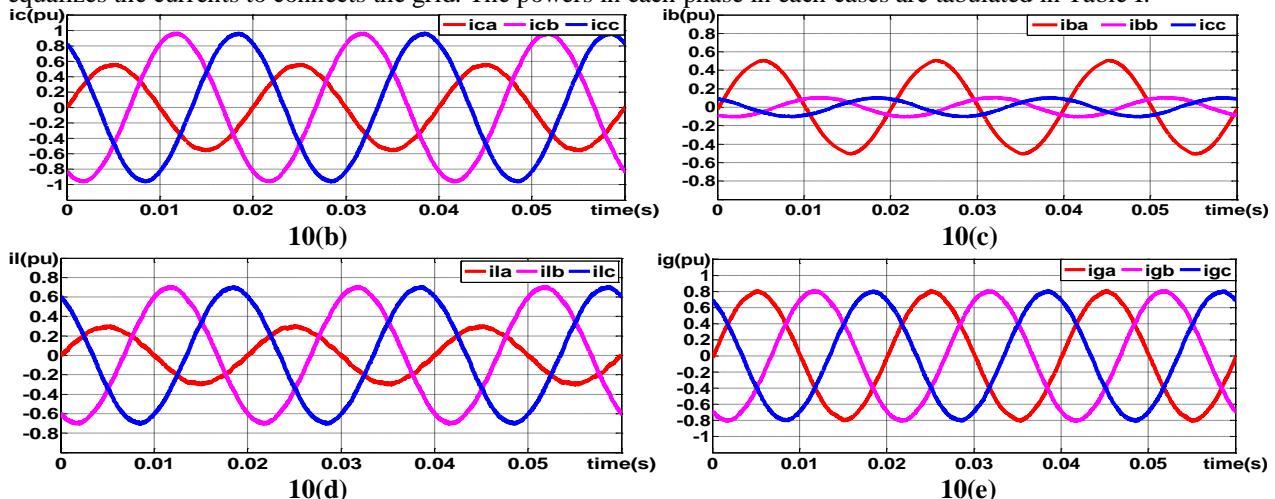
**Fig.10 Results with Parallel connection of BTB voltage source converter 10(b) 3-ph 7level CHB currents; 10(C) BTB converter currents; 10(d) Remaining currents  $i_{la}, i_{lb}, i_{lc}$ after the BTB consumed;10(e) Final grid currents  $i_{ga}, i_{gb}, i_{gc}$  in case C.**
