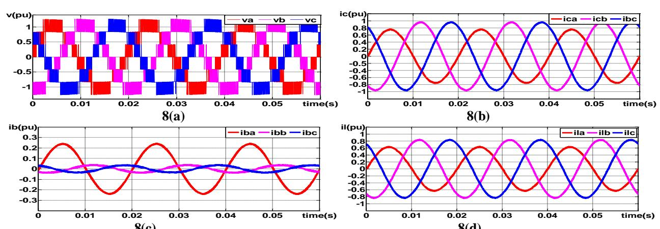
Fig.8 (a)&(b) 3-ph 7-level CHB converter voltages  $v_a, v_b, v_c$  and currents  $i_{ca}, i_{cb}, i_{cc}$ ; (c) BTB converter currents  $i_{aa}, i_{bb}, i_{bc}$ ; (d) Remaining currents  $i_{la}, i_{lb}, i_{lc}$  after the BTB consumed.
