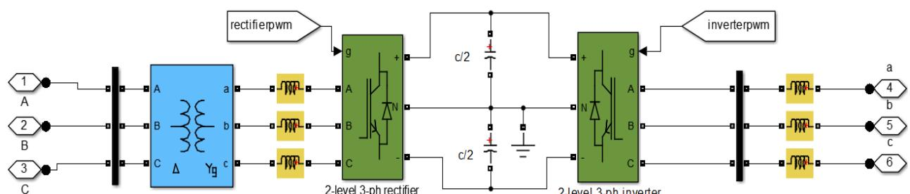
**Fig 2: Back to Back voltage source converter**
