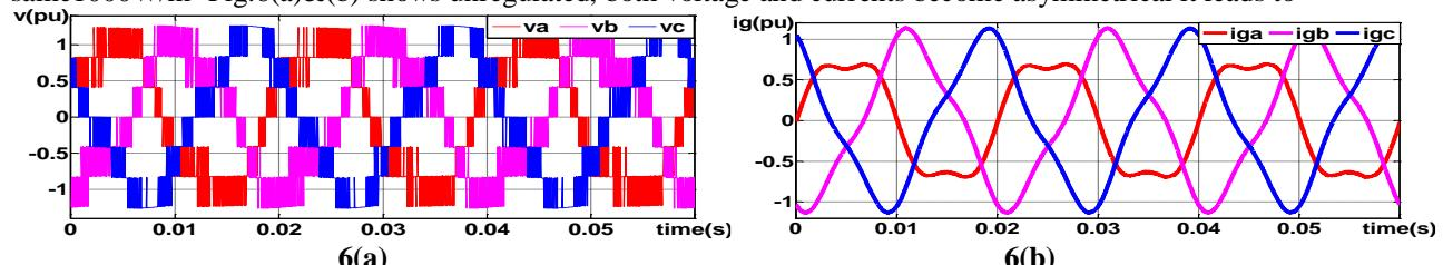
Fig.6 Unregulated with case B, a) 3-ph 7-level CHB converter voltages  $v_a, v_b, v_c$  and b) grid currents  $i_{ga}, i_{gb}, i_{gc}$
