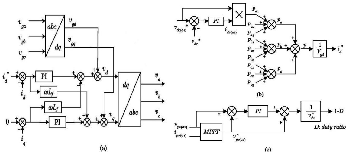
**Fig.3 Control implementation. (a) VOC of the CHB converter; (b) obtaining the current references; (c) MPPT regulation of the dc-dc converter**
