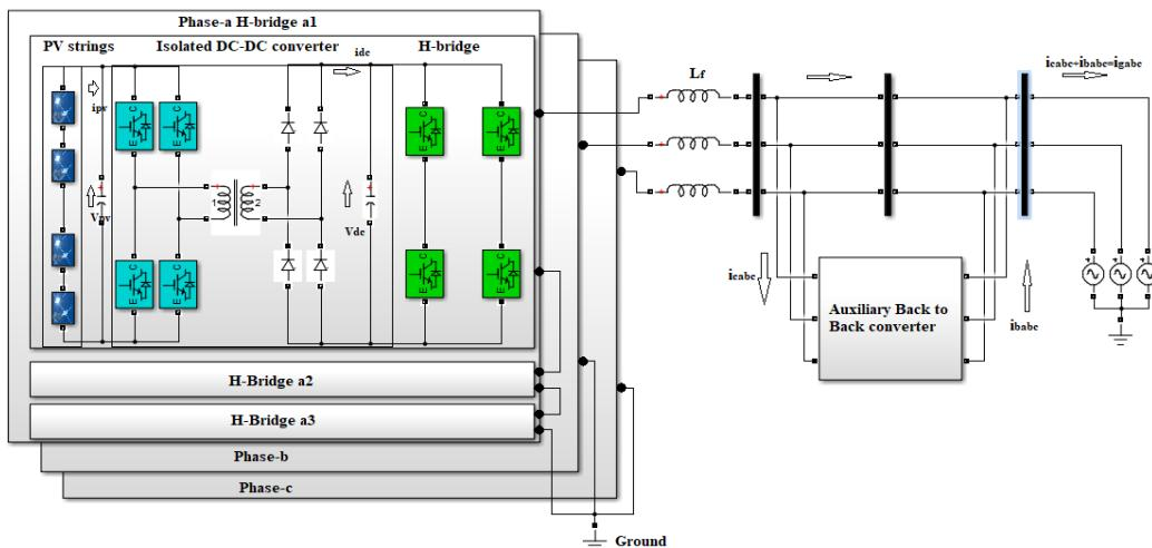
**Fig.1 Grid connected Three-phase seven-level cascaded H-bridge inverter with parallel connected Auxiliary back to back converter.**
