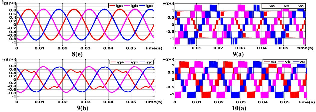
**Fig. 8(e) Final grid currents  $i_{ga}, i_{gb}, i_{gc}$  in case B; Fig.9 FFZSI regulated with case c 9(a)and9(b) 3-ph 7-level CHB voltages  $v_a, v_b, v_c$  and grid currents  $i_{ga}, i_{gb}, i_{gc}$ ; Fig.10(a) 3-ph 7-level CHB converter voltages  $v_a, v_b, v_c$ .**
