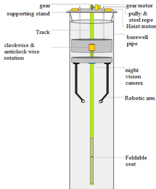
Fig 2: Rescue device setup
