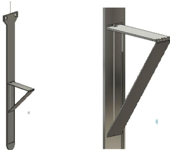
Fig 4: The supporting foldable arm
