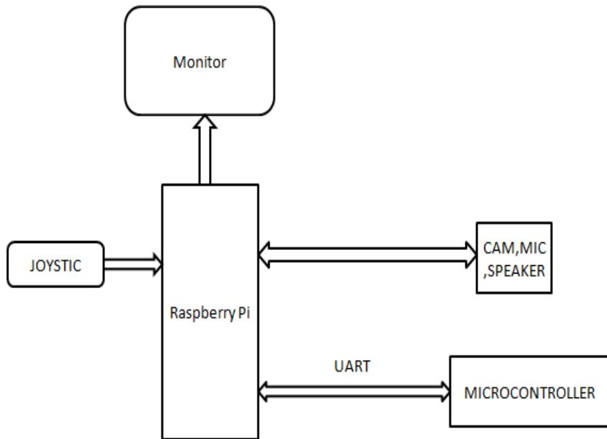
Fig 5: Transmitter module
