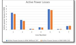
Fig (21): Active power losses in the system with SVC
