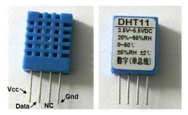
Figure 3: Temperature and Humidity Sensor
