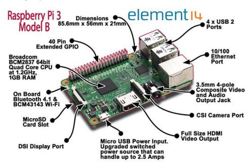
Figure 2: Raspberry Pi 3 Module Description
