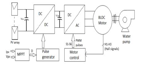
Figure 1. Block diagram of a solar water pump using BLDC motor III. DESIGN TOPOLOGY
