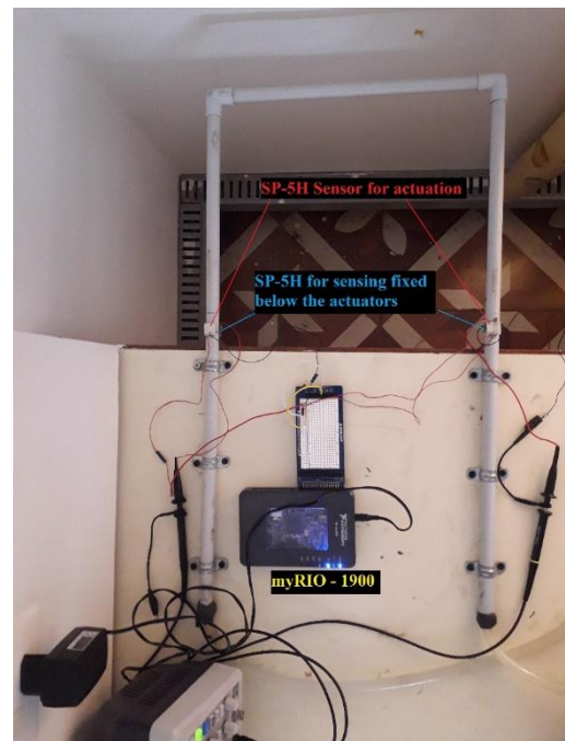
Figure: 5 PZT patches placement on the CMF model for frequency analysis.
