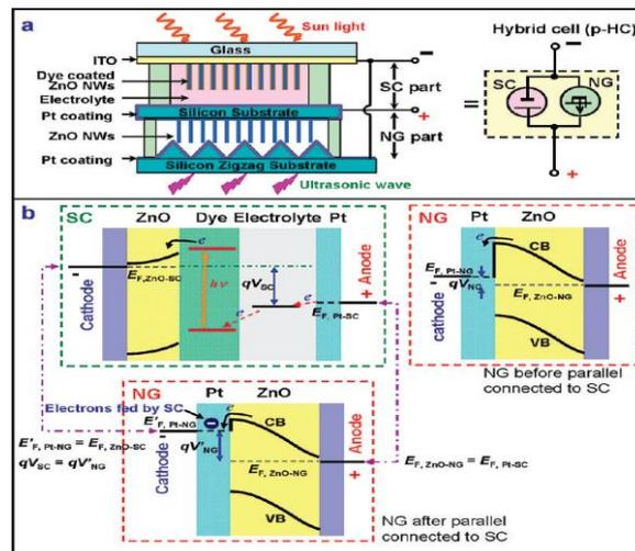
**Figure 3:** Design of a hybrid cell composed of parallel integrated solar cell and nanogenerator for raising the output current. (a) Schematic structure of the HC design. The central Pt-coated silicon substrate is defined as the anode, and the ITO layer electrically integrated to zigzag electrode is defined as the cathode of the HC. A symbol of the HC
