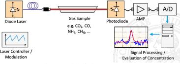
Fig.3Tuneable diode spectroscopy.
