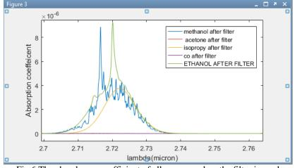
Fig.6 The absorbance coefficient of all gaseous when the filter is used
