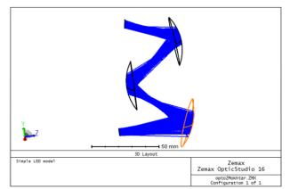
Fig. 13 3D layout of the design shows how the reflective concave mirrors are arranged.
