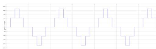
Figure.6. Five level output waveform for FC-MLI
