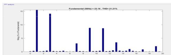
Figure.10.FFT analysis of diode clamped inverter
