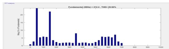
Figure.7. FFT analysis of clamping capacitor inverter
