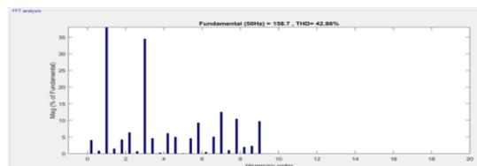
Figure.5. FFT analysis of diode clamped inverter
