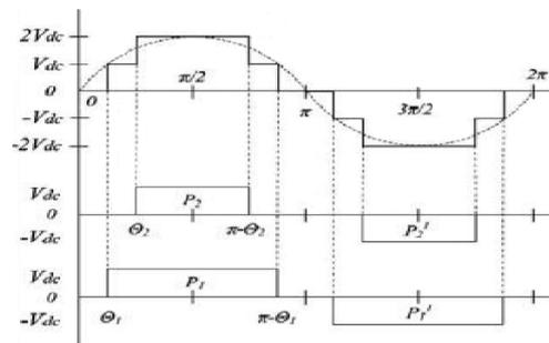
Figure.3. Five level output waveform
