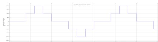
Figure.9. Five level output waveform for CHB-MLI
