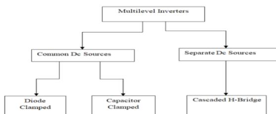
Figure.1. Topology for multilevel inverter
