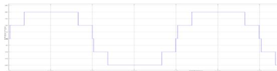
Figure.4. Five level output waveform for DC-MLI
