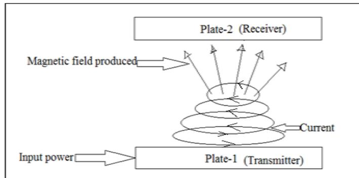
**FIG 1: GENERAL DIAGRAM OF TRANSMITTING AND RECEIVING PLATE**
