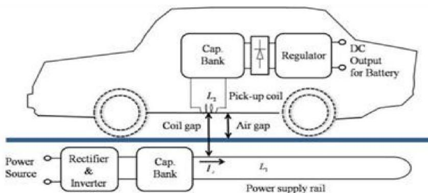
Fig 5 :Roadway powered electric vehicle.
