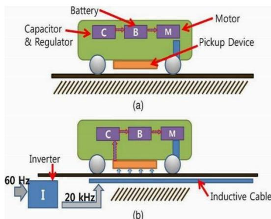
**Fig. 3:** (a) WPT without transmitters (b) WPT with transmitters[14]
