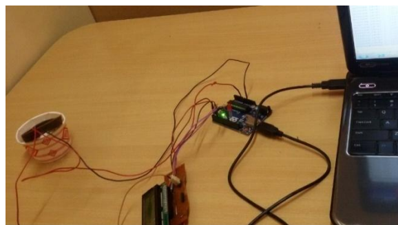
Fig. 9 Moisture Sensor is Interfaced in the Microcontroller
