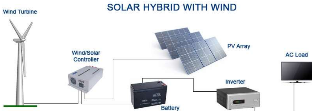
FIG 3: SCHEMETIC DAIGRAM OF WIND SOLAR GENERATION
