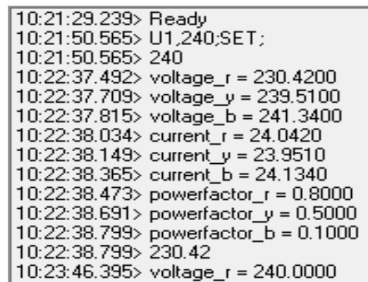
Fig. 9: Terminal software display for setting required source value and for logging data
