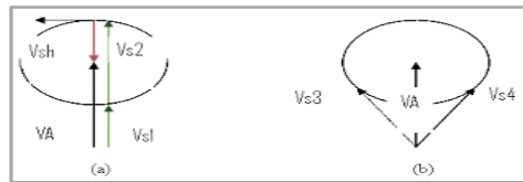
Fig. 2 Power exchange of the Shunt Converter
