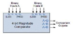
It can compares two 4 bit binary number Aand B and the outcome of comparator has been specified by three binary variables G(A>B), E(A=B), E(A=B).
