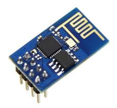
Its high degree of on chip integration allows for minimal external circuitry, including the front end module, is designed to occupy minimal PCB area. One useful feature of Uno Wi-Fi is support for OTA(over the air) programming, either for transfer of arduinosketches or Wi-Fi firmware. The ESP8266 is capable of either hosting an application or offloading all Wi-Fi networking functions from another application processor.
