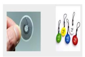
In order to power these NFC tags, electromagnetic induction is used to create a current in a passive device.
