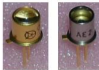
Fig7: (Left) OPTEK OP232 IRLED. (Right) Centronic BPX65 photodiode
