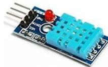
Fig 3:DHT11 Sensor
