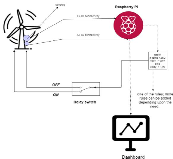
Fig 1:Schematic diagram of the proposed system
